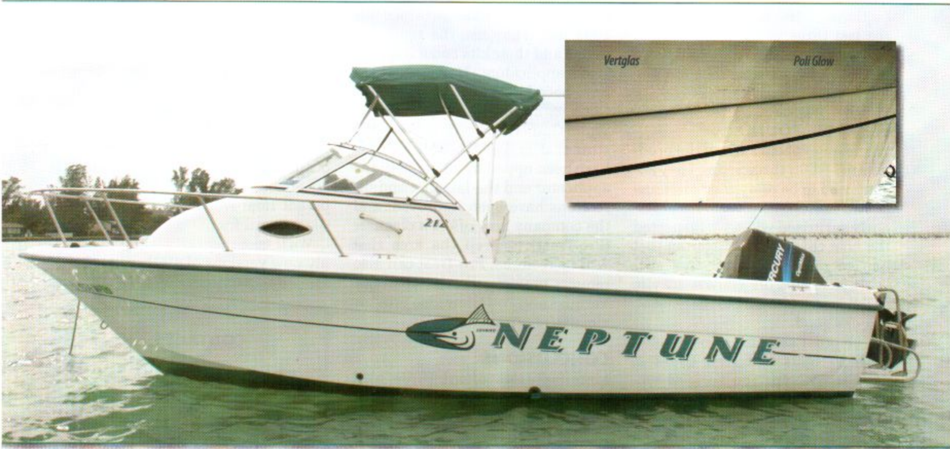
In 2003, testers coated this boat's hull with three hull restorers: Poli Glow (bow), Vertglas (amidships), and New Glass 2 (aft and stern). Poli Glow's sheen (above) and water-beading action (inset right) are still visible on the boat's bow.
